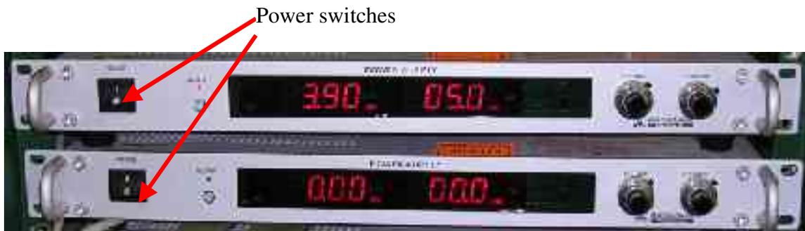
**Figure 1. Primary High-Voltage power supplies**
